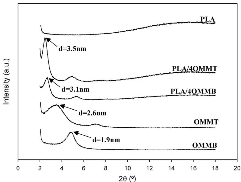
Figure 1 WAXD patterns curves for OMM nanoclays, PLA/4OMM nanocomposites and PLA.
