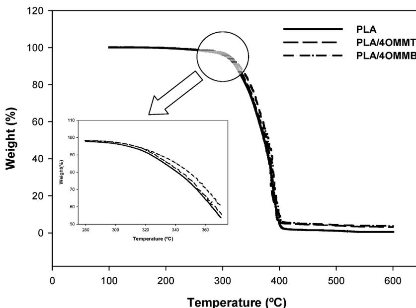
Figure 3 TGA curves for pure PLA and PLA/4OMM nanocomposites.
